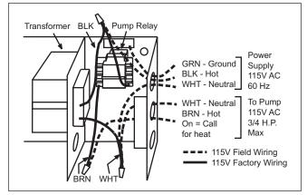
Figure 8. Field Wiring Connections.
